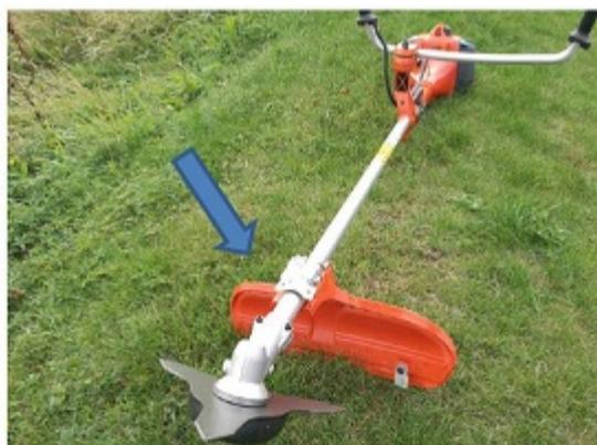
Protective guard fitted incorrectly
