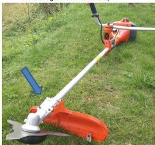
Protective guard fitted correctly
