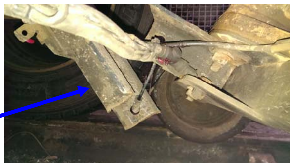
The failed front nearside arm that connects the rail axle to the vehicle chassis.
