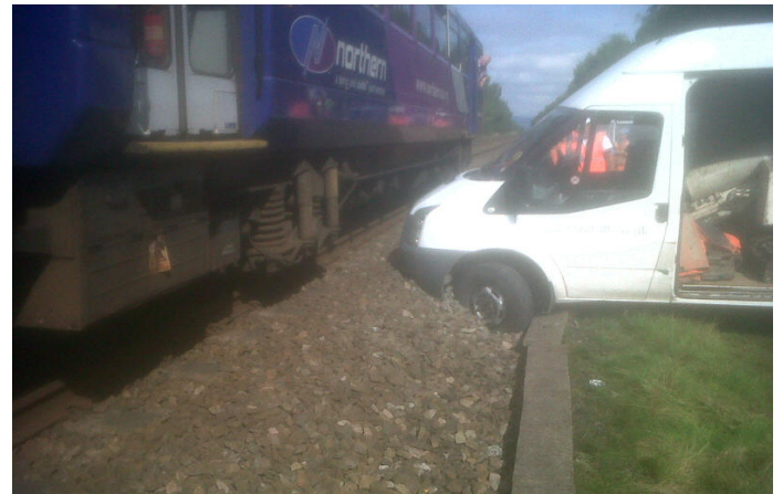
Vehicle within 1 metre of an operational line
